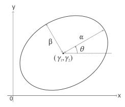
The **label**, the semi-major axis  $\alpha$ , the semi-minor axis  $\beta$ , the *x*-coordinate  $\gamma_1$  and *y*-coordinate  $\gamma_2$  of the centre  $(\gamma_1, \gamma_2)$ , and the angle of rotation  $\theta$  of the three ellipses must be defined (one line for each ellipse). The ellipses must be labelled as **a**, **b**, **c**.
